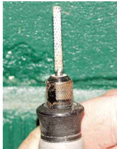
Close up of diamond grinder No 562, which works well for cutting and beveling camelid teeth. Choosing the correct cutting device is essential to successfully cutting teeth. If the wrong head is used the cut may take an inordinate amount of time, chip the teeth and cause undue stress to the animal and undermine the integrity of its teeth. Also prolonged cutting makes restraint more difficult as the animal fights to avoid discomfort. The selection of the correct cutting bit is extremely important for animal welfare and precision work.
